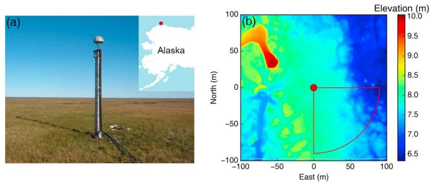
**Figure 1.** (a) Ground photo viewing the GPS station SG27 toward east on 24 August 2010 (Photo: UNAVCO). The inset shows the location of Barrow (red circle) in Alaska. (b) Relief map of the area surrounding SG27 (marked by the red circle). The red wedge outlines the footprint of the reflected GPS signals.
