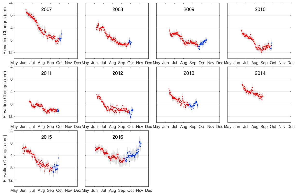
**Figure 2.** Time series of daily elevation changes on snow-free days from 2007 to 2016. The red dots and blue dots represent the thaw and freezing seasons, respectively. The gray error bars represent the uncertainties of the elevation changes. The 2016 time series is identical to those shown in Figures 3a and 4b.
